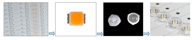
PCB + CHIP(step 1) + LENS(step 2) = Finish
